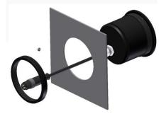
Attention! Chek the sealing O-Ring between the lamp and the support surface.
